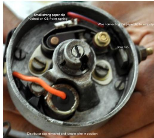
Distributor with jumper connected.
