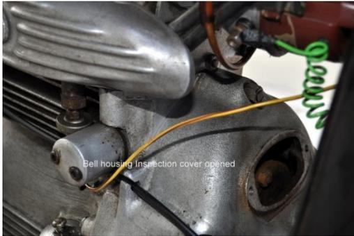
Bell housing- Inspection door removed
